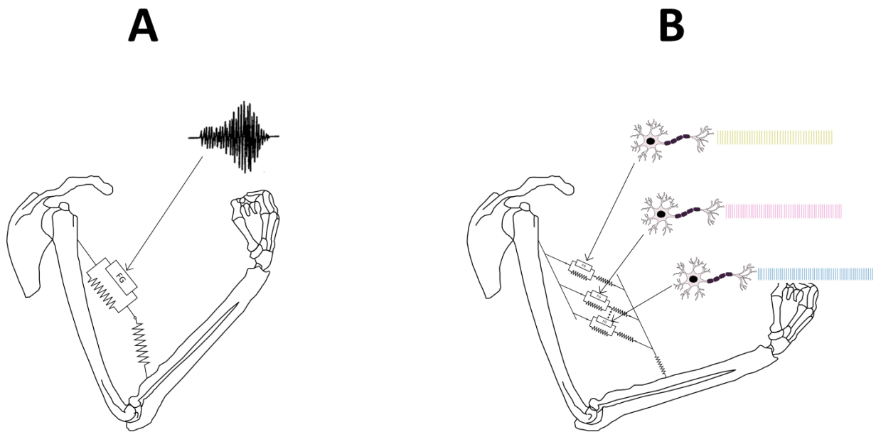
Figure 1-1: Description of a whole muscle with Hill-type actuators. Hill-type models typically include two passive spring-like elements to account for the passive properties of the muscle-tendon tissue, and a force generator (FG) that describes the active neuromechanical dynamics of the muscle tissue. (A) A unique Hill-type model is used to describe the muscle's macroscopic properties responsible for force generation. It is driven by a unique neural control, that is obtained from processed bipolar EMG signals in bEMG-driven methods. (B) The whole muscle is described as a collection of in-parallel Hill-type actuators that describe the neuromechanical dynamics of individual MUs. The muscle is driven by multiple neural controls, that are the MN spike trains obtained from processed HDEMG signals, three of which are represented here. Methods for developing such MN-driven multi-MU neuromuscular model are proposed in this thesis.
